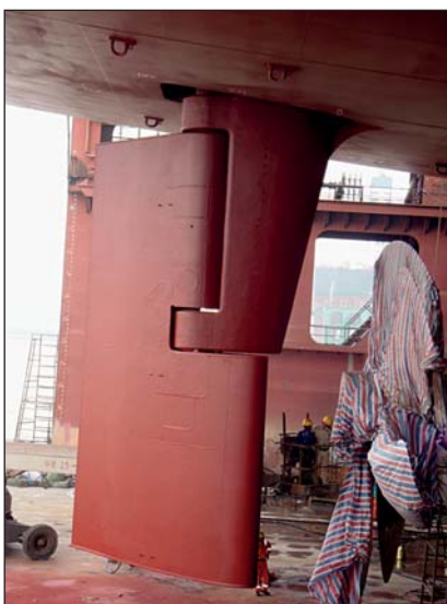
Ecospeed is applied in only two, identical layers.
