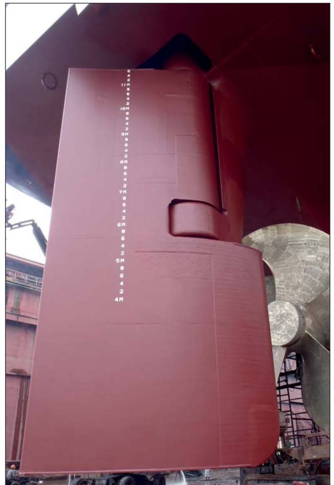
Ecospeed can protect a rudder against the forces produced by cavitation.
