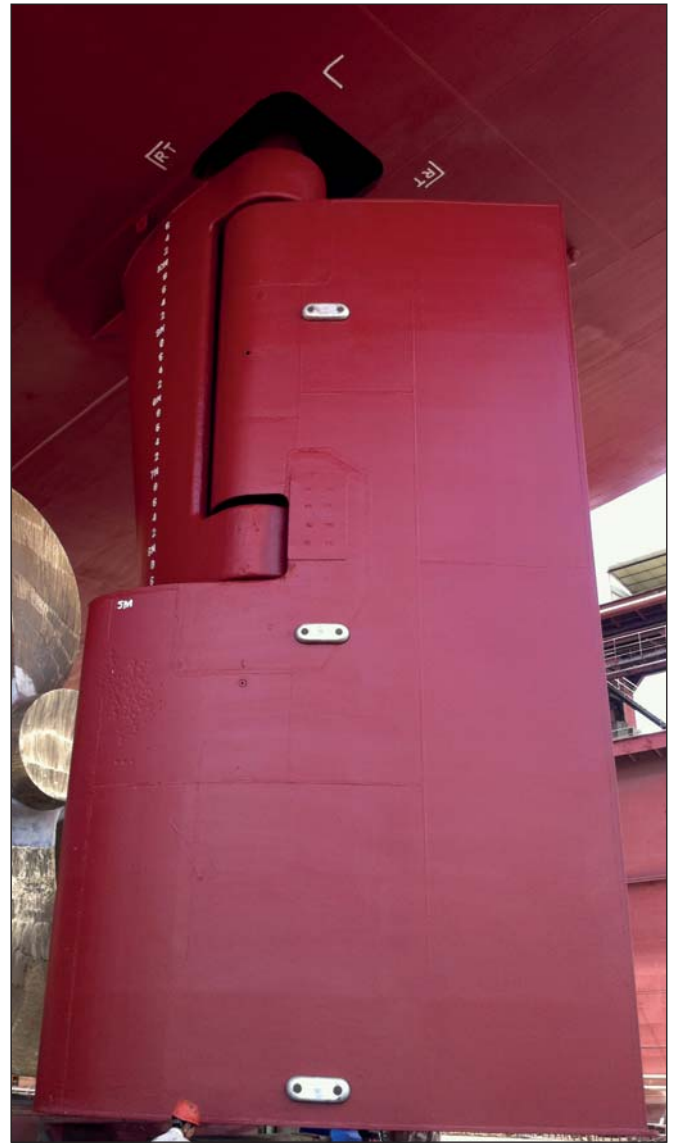
Ecospeed will protect the rudder against cavitation and corrosion damage.
