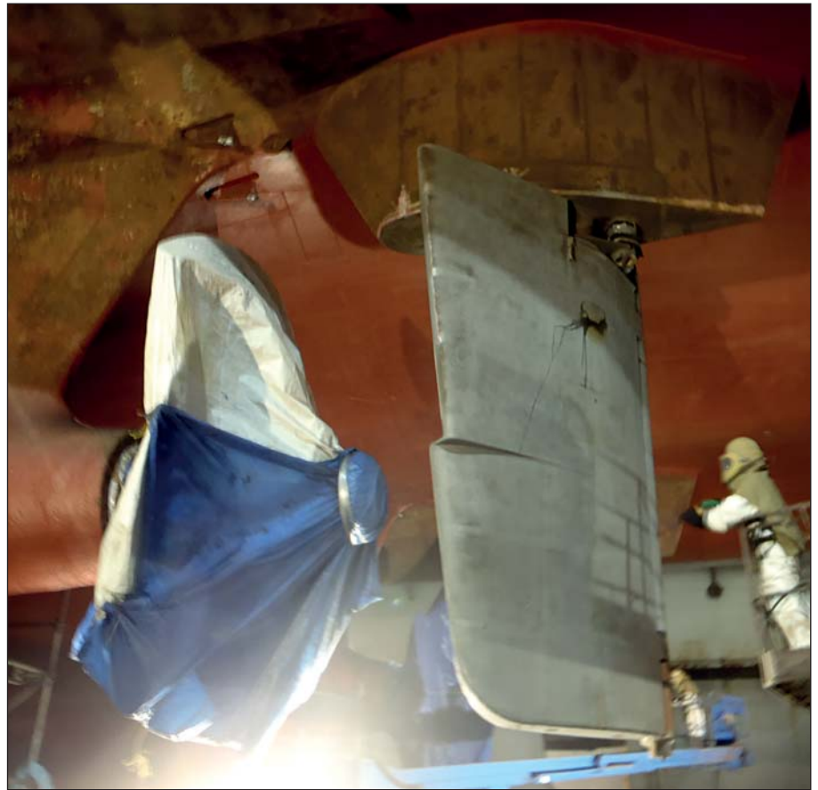
After surface preparation, Ecospeed is applied in two identical layers.
