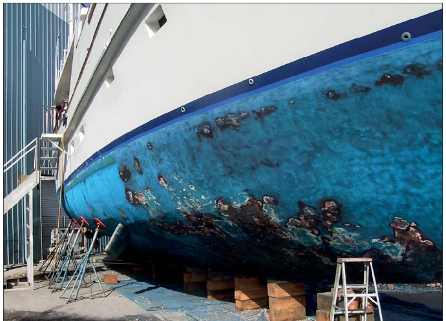
Detail of the condition of the hull in 2007 prior to Ecospeed application.
