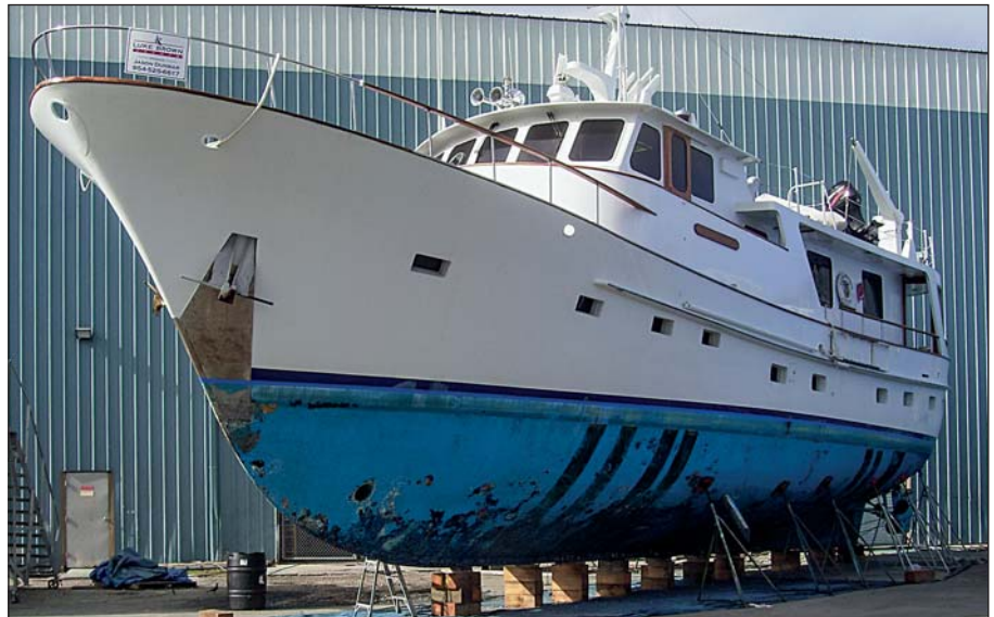
The Oceantide out of the water just before the hull was grit blasted and Ecospeed was applied.
