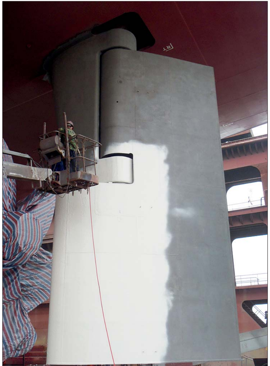
Application of first layer of Ecospeed on rudder in Shanghai.
