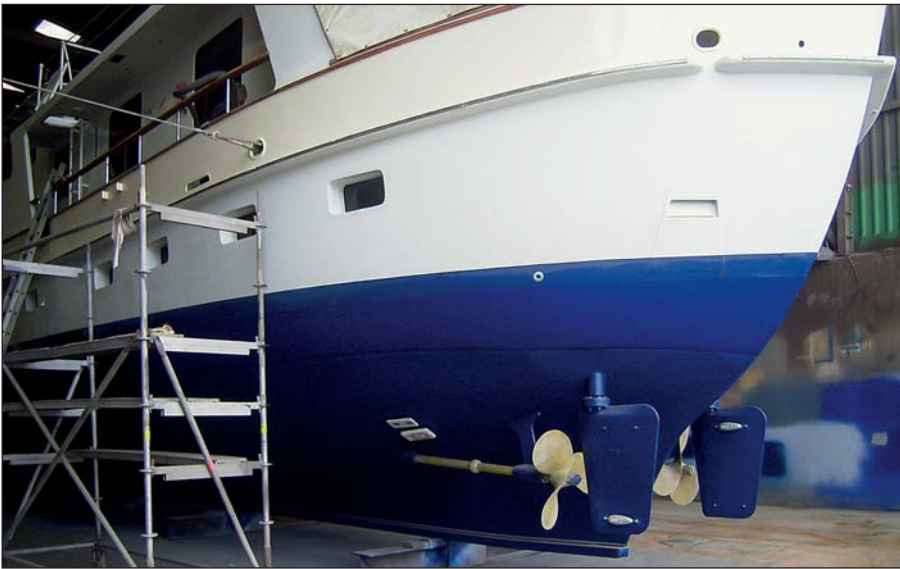
Newly applied Ecospeed on the hull.
