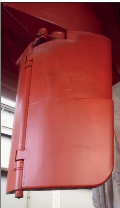
Ecospeed will protect the rudder for the remainder of the vessel's service life.
