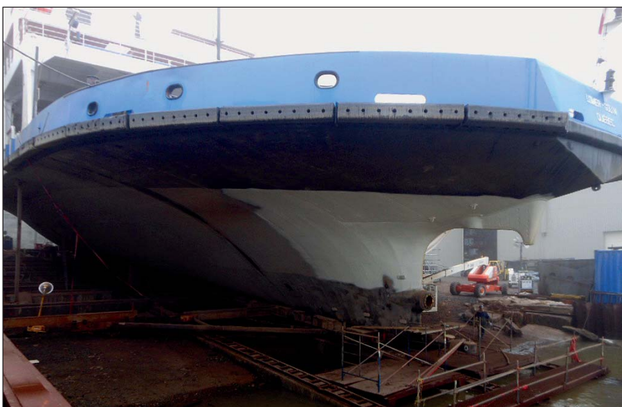
The ice class ferry in drydock during Ecospeed application.
