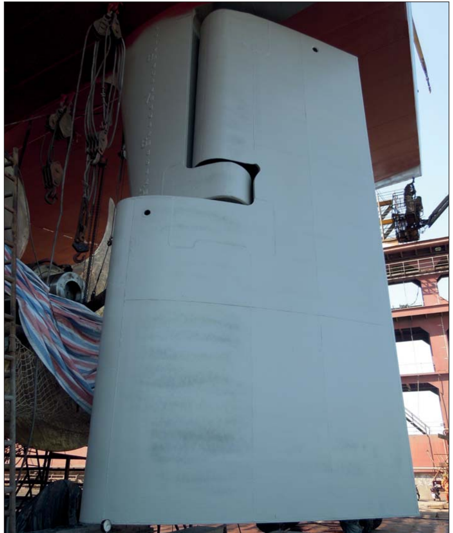
Ecospeed is applied in two identical layers.
