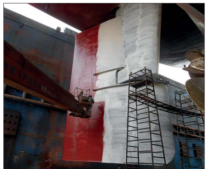
Application of second layer.
