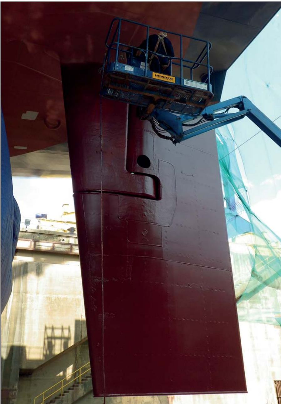
Ecospeed will protect a rudder against cavitation and corrosion damage.
