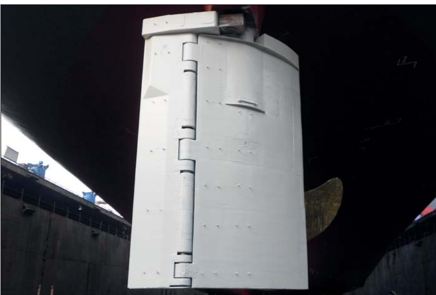
Ecoshield will protect a rudder against cavitation damage.
