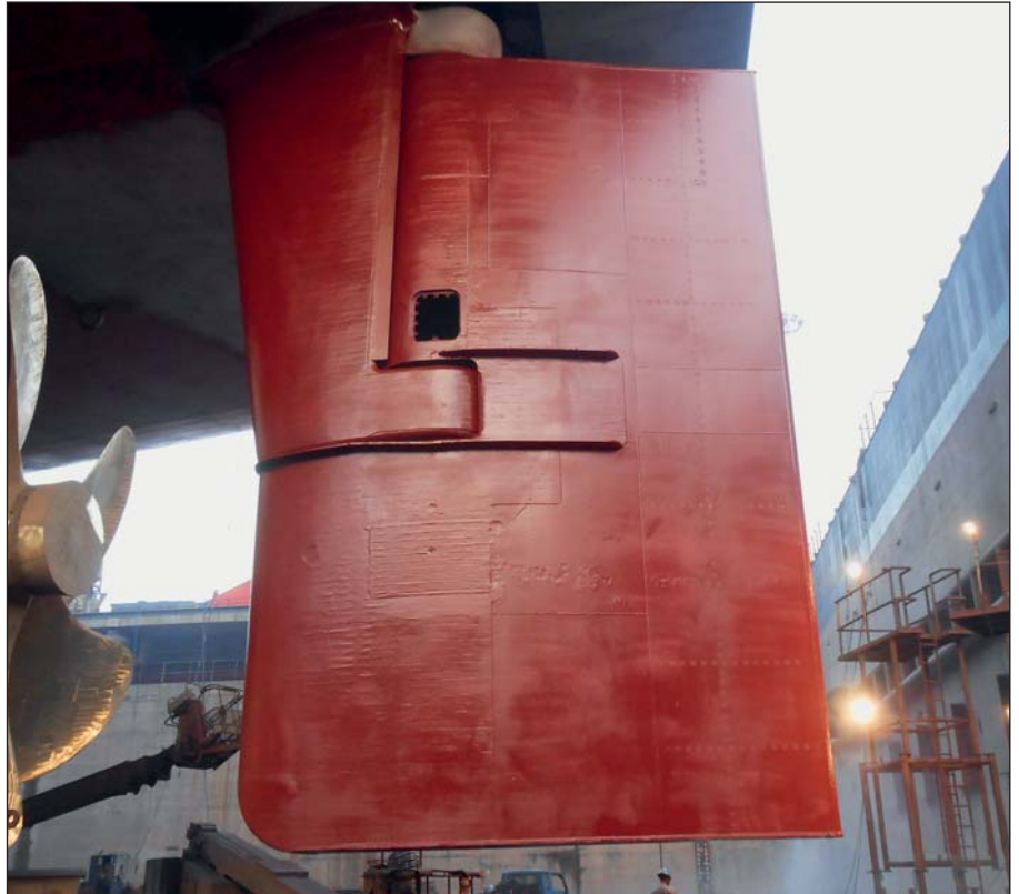
Ecoshield is applied in two identical layers.
