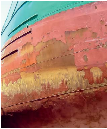
General cargo ship, before Ecospeed, one season trading in Baltic ice.
