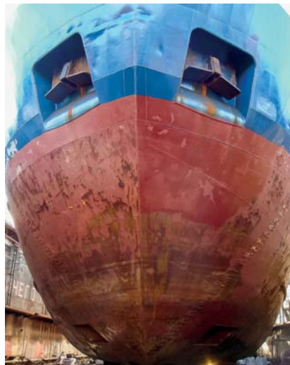
Hull of ice-going general cargo ship after a season in ice, eight years after launch with annual coating repair or replacement.
