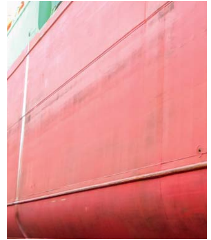
Same ship, same conditions, five years after Ecospeed applied, no repaint.
