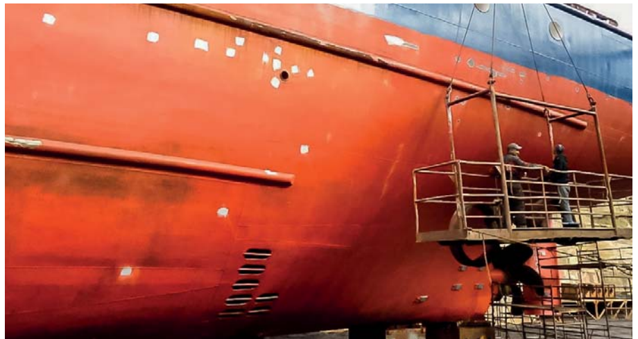
Five years after Ecospeed applied, the same hull is still smooth and the coating intact, requiring only minimal touch-ups in drydock despite trading in icy waters and no coating repair since application.
