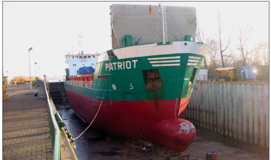
Only touch ups required on ice-going general cargo vessel after 5 Baltic winters with Ecospeed
