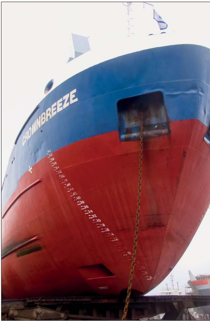
Crownbreeze in drydock in 2009 showing condition of paint after two years in ice.
