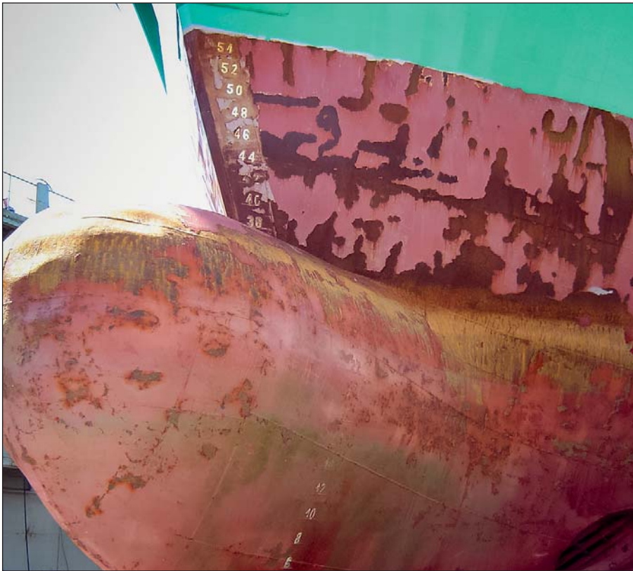
MV Patriot in drydock in 2005, prior to blasting and Ecospeed application.
