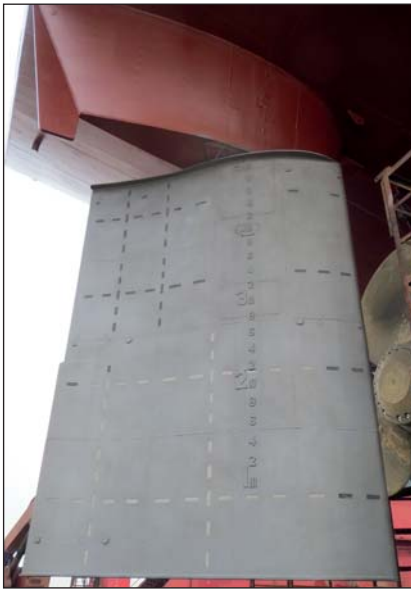
After surface preparation, Ecoshield is applied in two layers.
