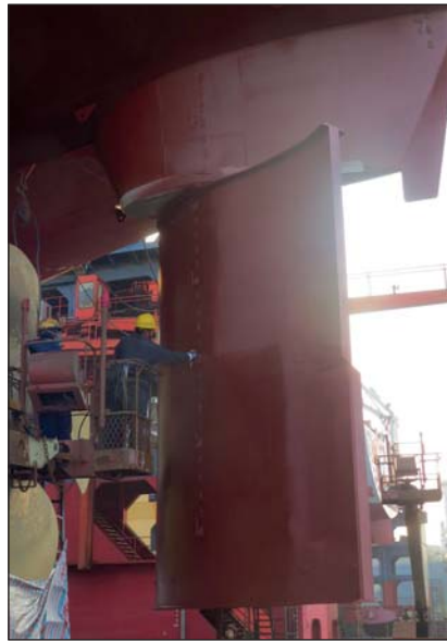
Application of second layer on general cargo vessel's rudder.
