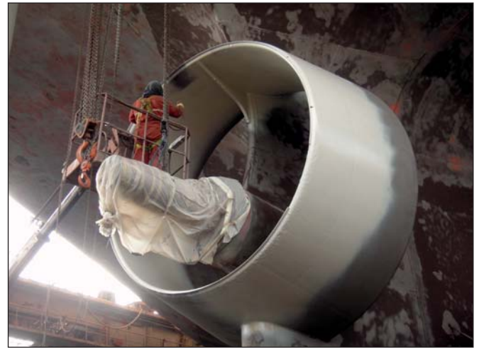
Ecoshield was applied on the nozzles of two container vessels.
