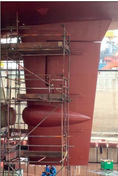
Ecoshield will protect this rudder for the rest of its service life.
