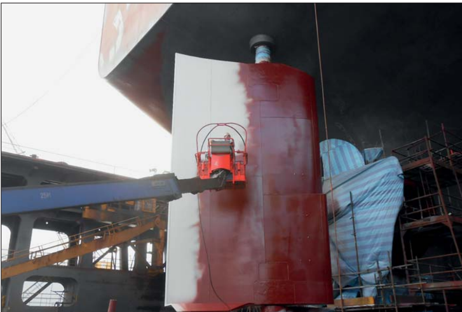
Ecoshield is applied in only two layers.
