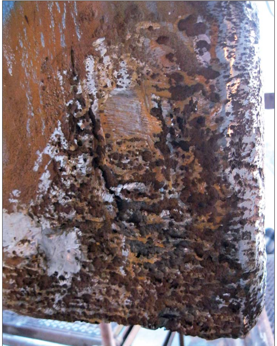
Severe cavitation damage on rudder prior to Ecoshield application.
