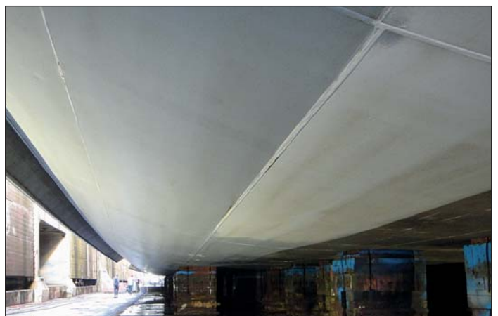
This cruise ship came out of the water just like this. The Ecospeed coating is 5 ½ years old. It has had absolutely minimal touch-ups, no repair, no replacement. It has undergone routine in-water cleaning. The ship gained two knots over trial speeds when the coating was changed to Ecospeed.
