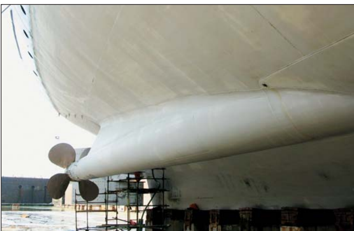
This cruise ship came out of the water just like this. The Ecospeed coating is 5 ½ years old. It has had absolutely minimal touch-ups, no repair, no replacement. It has undergone routine in-water cleaning. The ship gained two knots over trial speeds when the coating was changed to Ecospeed.
