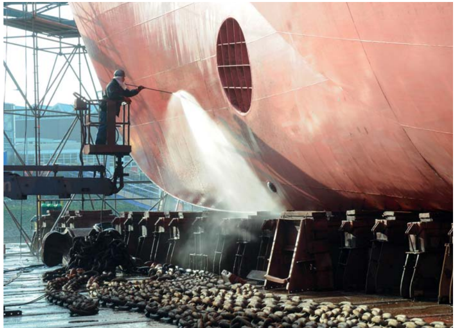
Fouling can be removed in drydock with high pressure tools or underwater while improving the coating.
