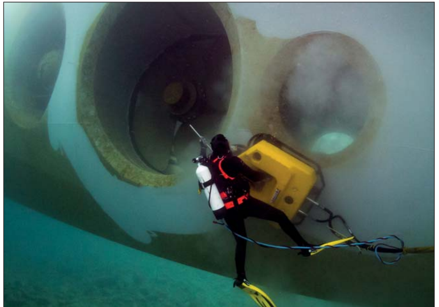
Routine in-water cleaning keeps this cruise ship's Ecospeed coated hull clean. In fact Ecospeed gets a little smoother with each cleaning. And the cruise line is saving at least 10% on fuel costs (compared to when it was using TBT).
