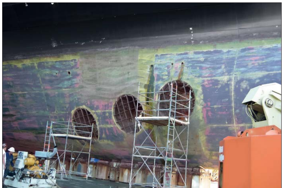
Cruise vessel's toxic SPC coating showing paint degradation.
