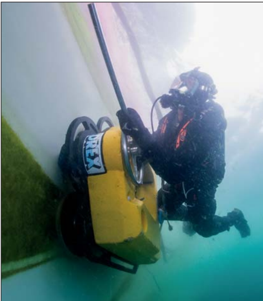
Routine in-water cleaning keeps this cruise ship's Ecospeed coated hull clean. In fact Ecospeed gets a little smoother with each cleaning. And the cruise line is saving at least 10% on fuel costs (compared to when it was using TBT).
