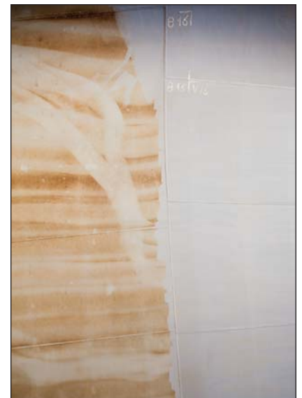
Fouling on Ecospeed can be removed fast and easy.
