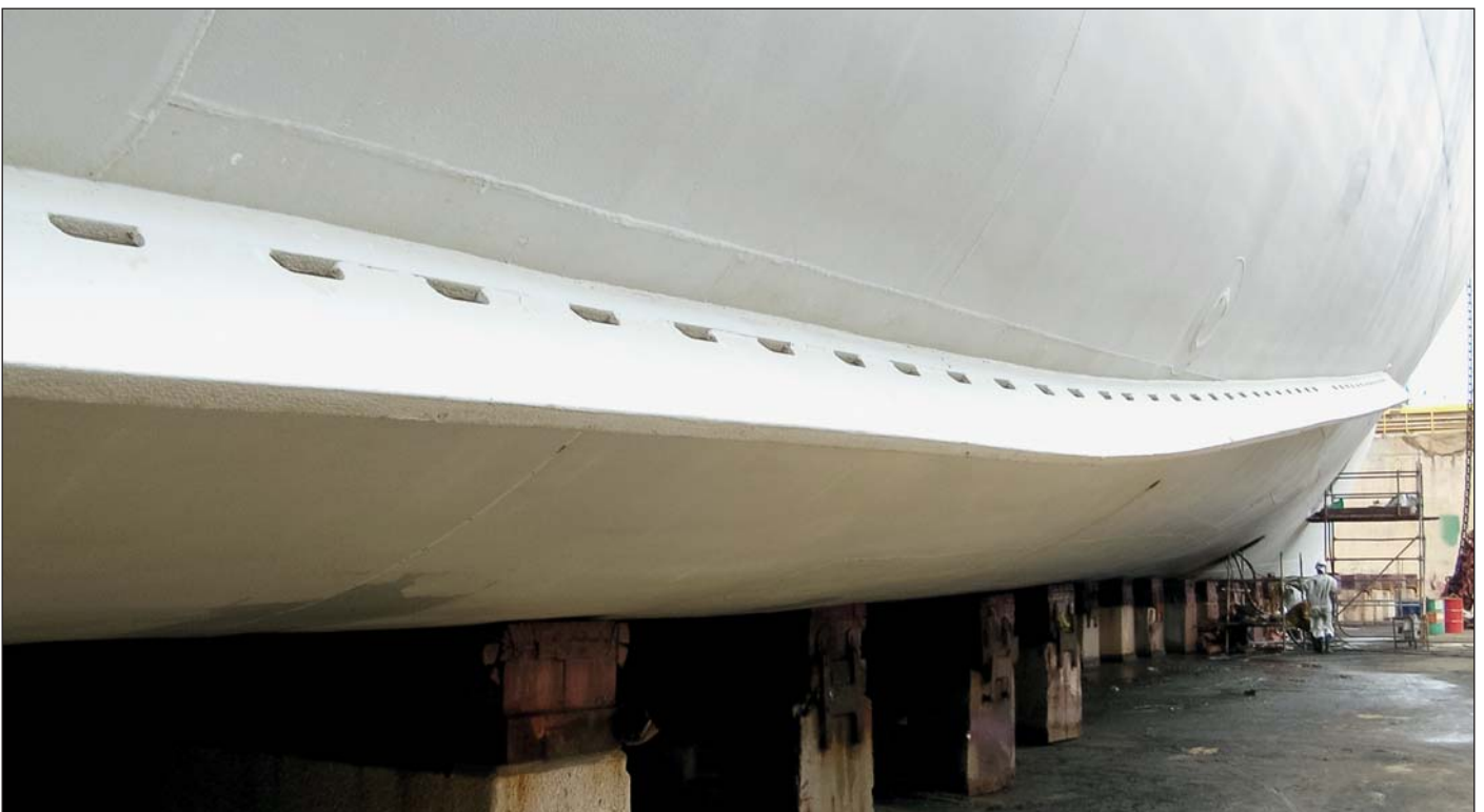
Routine in-water cleaning keeps this cruise ship's Ecospeed coated hull clean. In fact Ecospeed gets a little smoother with each cleaning. And the cruise line is saving at least 10% on fuel costs (compared to when it was using TBT).
