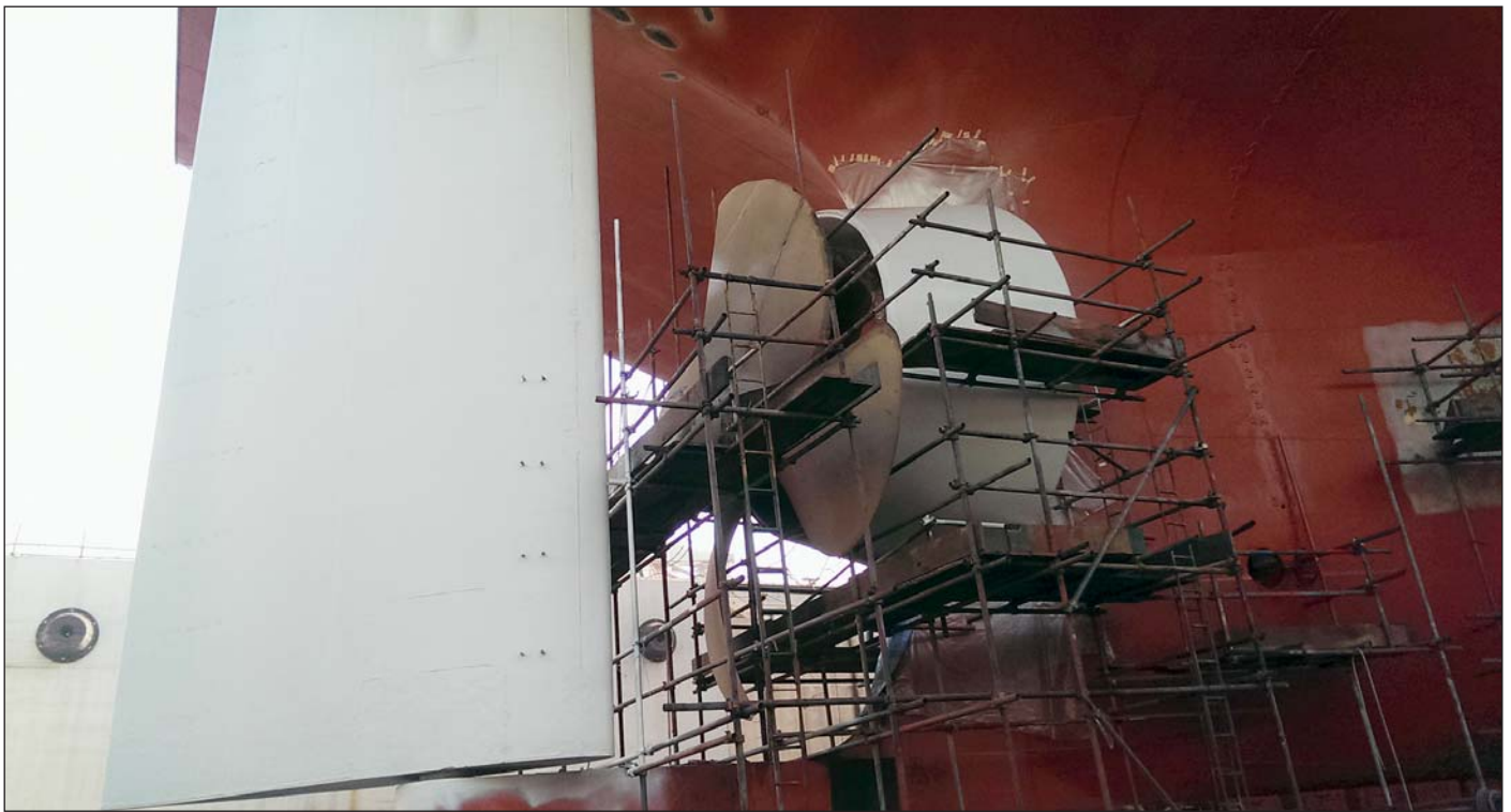
Rudder and nozzle after application of first layer.
