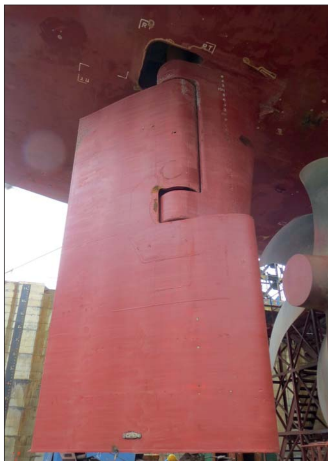
The same rudder after sailing with Ecoshield for five years.
