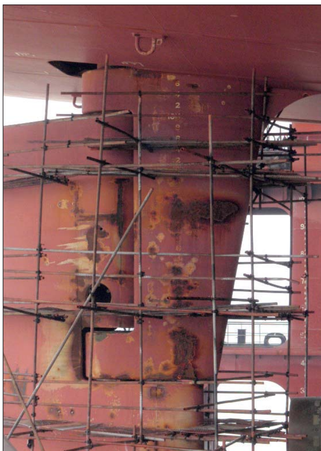
Rudder of container vessel after sailing with traditional coating system.
