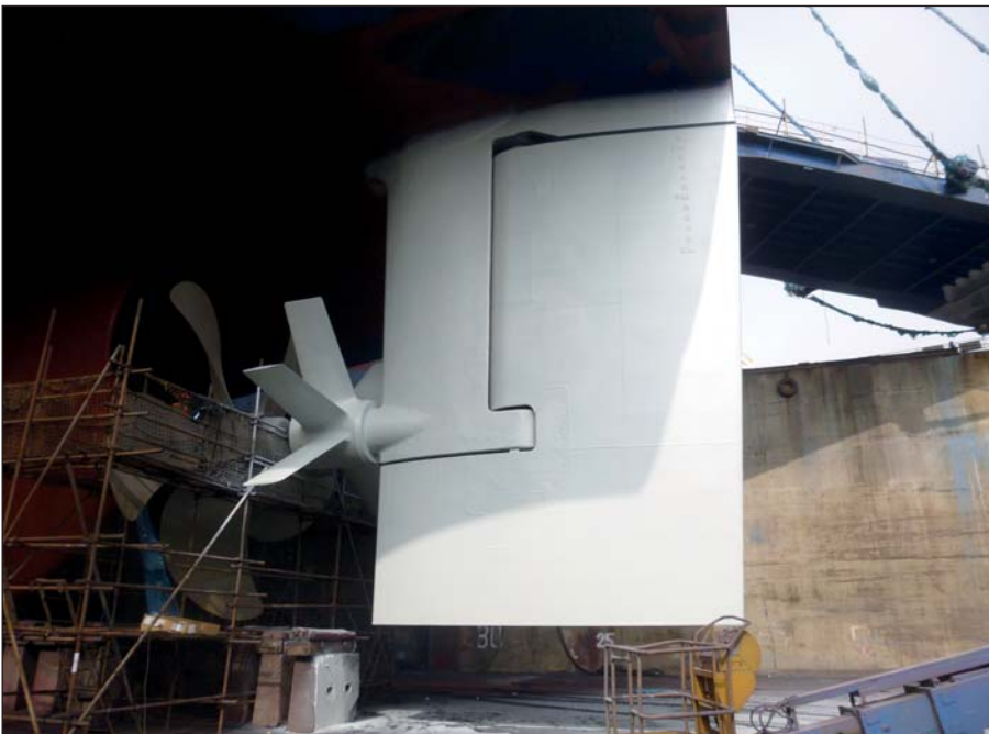
Overcoat time between layers can be as short as three hours.
