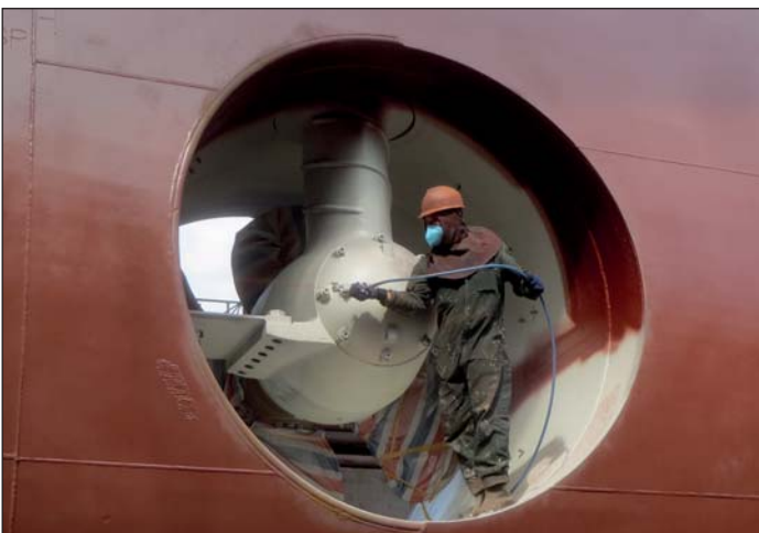
Thruster tunnels and other running gear is given a lifelong protection with Ecoshield.
