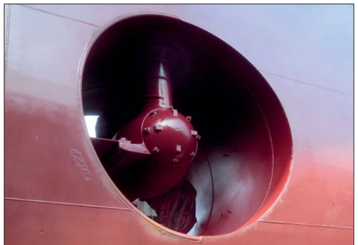
Thruster tunnels and other running gear is given a lifelong protection with Ecoshield.
