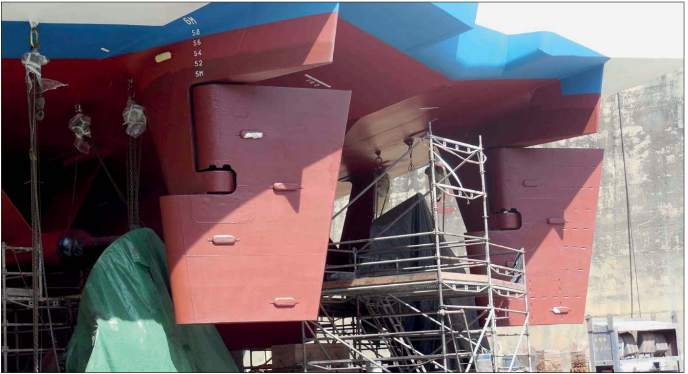
Both rudders of this passenger vessel were coated with Ecoshield in France.
