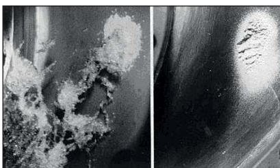
Cavitation bubbles and resulting damage.
