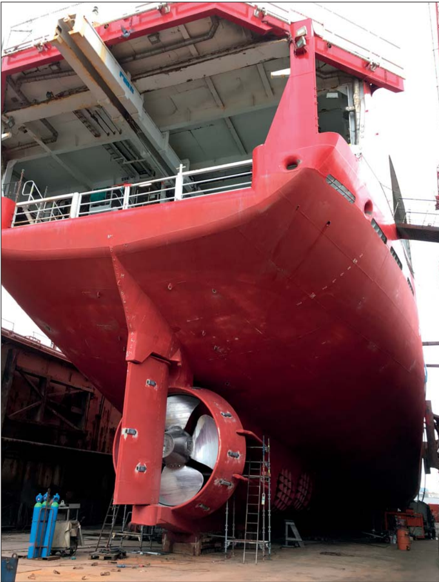
In eight seasons operating RRS Ernest Shackleton with Ecospeed coating, only those areas most susceptible to ice impact needed touch-ups.
