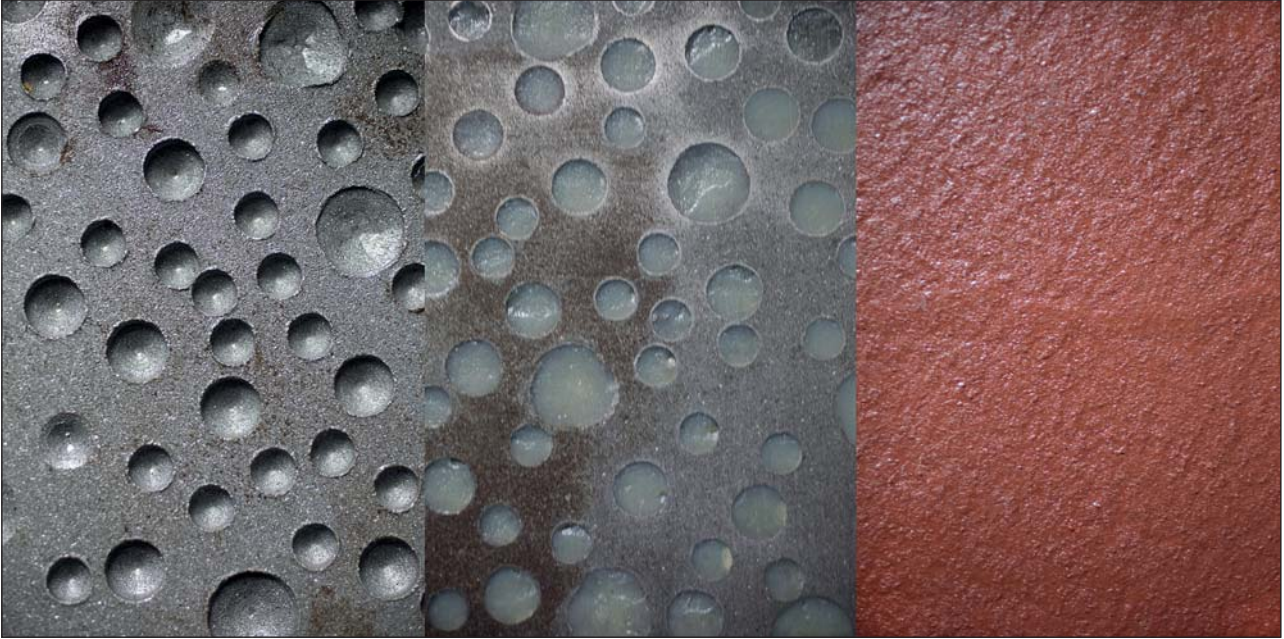
Test plate showing the benefit of an Ecofix and Ecoshield combination.
