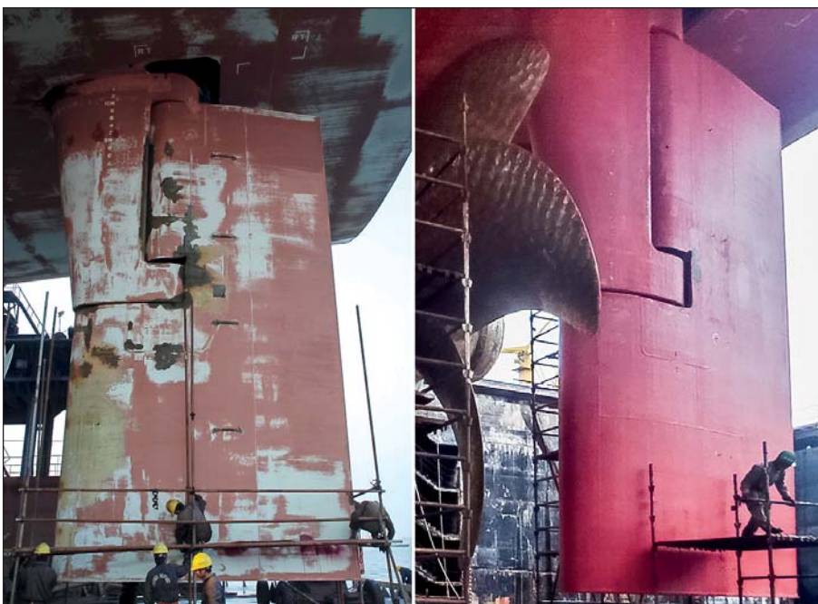
The rudder of the Maersk Deva after five years in service with conventional rudder coating (left), and five years after Ecoshield glassflake rudder coating was applied.
