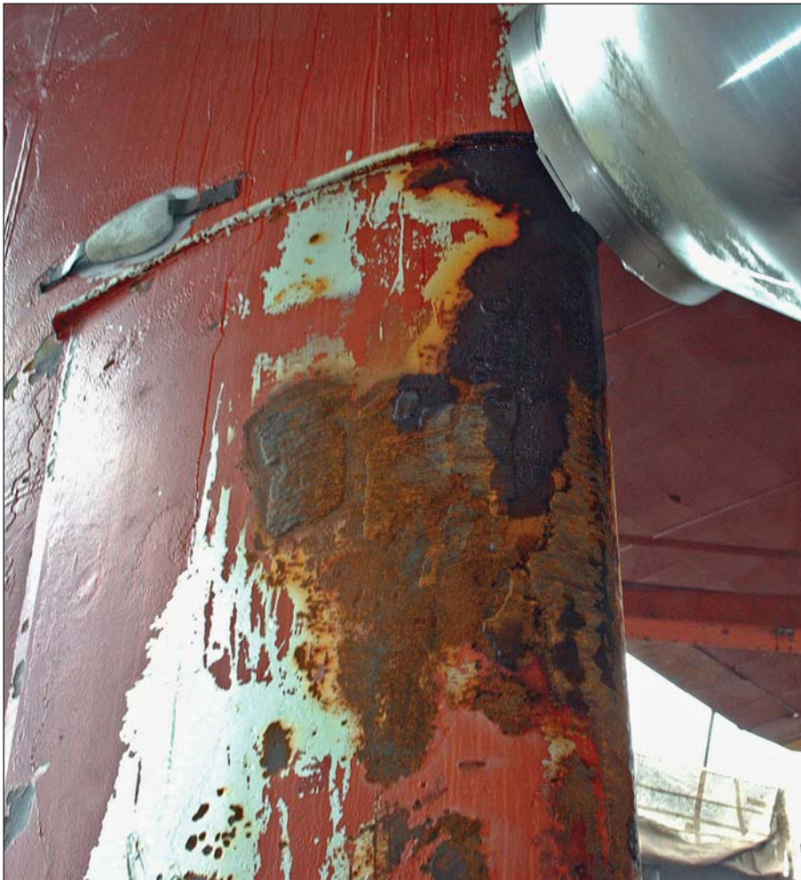
The damage caused by cavitation (left) and a typical welding repair (right).
