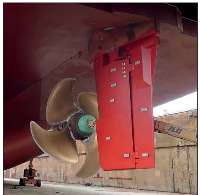
Ecoshield gives lasting protection against corrosion and cavitation damage.
