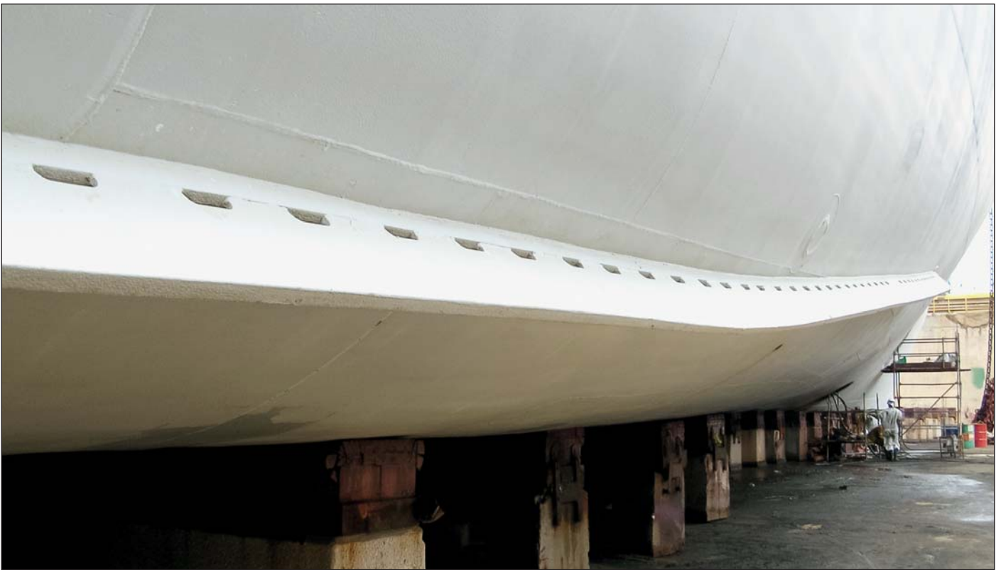
Routine in-water cleaning keeps this cruise ship's Ecospeed coated hull clean. In fact Ecospeed gets a little smoother with each cleaning.
