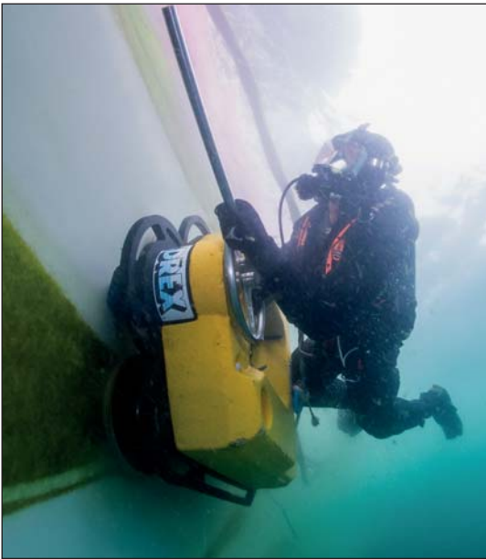
Routine in-water cleaning keeps this cruise ship's Ecospeed coated hull clean. In fact Ecospeed gets a little smoother with each cleaning.
