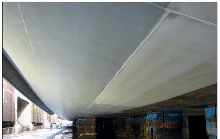
This cruise ship came out of the water just like this. The Ecospeed coating is 9 years old. It has had absolutely minimal touch-ups, no repair, no replacement. It has undergone regular routine in-water cleaning.
