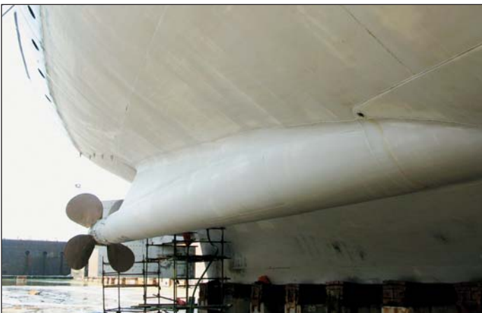
This cruise ship came out of the water just like this. The Ecospeed coating is 9 years old. It has had absolutely minimal touch-ups, no repair, no replacement. It has undergone regular routine in-water cleaning.
