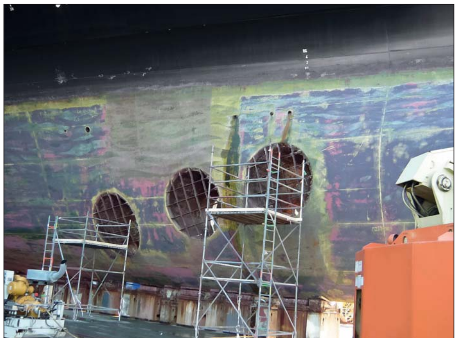
Cruise vessel's toxic SPC coating showing paint degradation.
