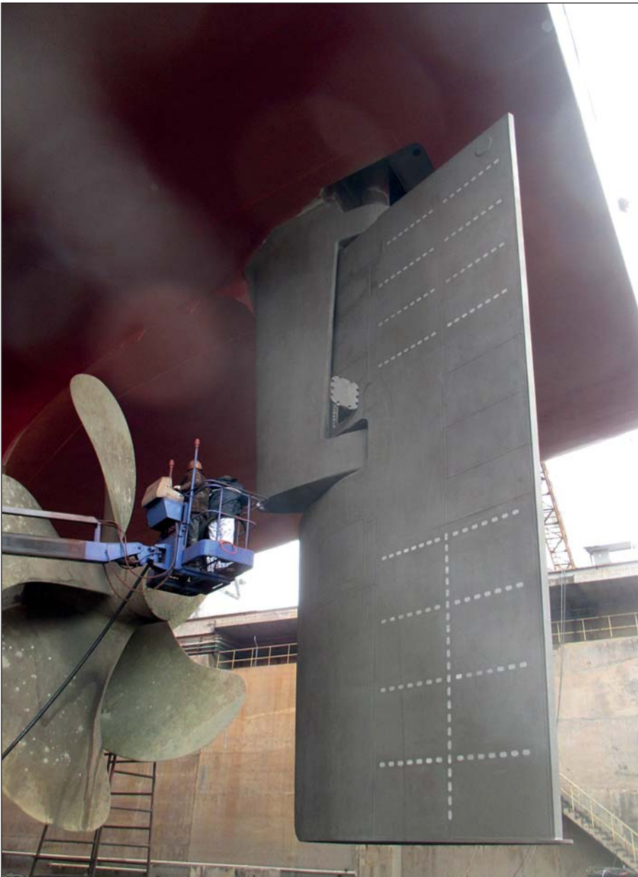
All existing paint layers are removed to start with a clean slate.
