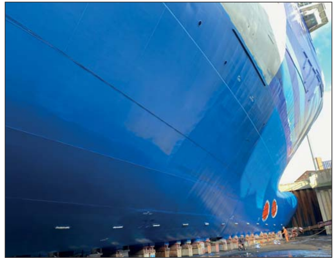
The durability of Ecospeed makes the planning of future dockings far easier.
