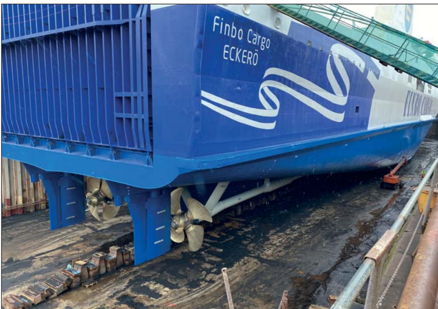
Most of the underwater hull was coated with Ecospeed to make sure no repaint would be needed.
