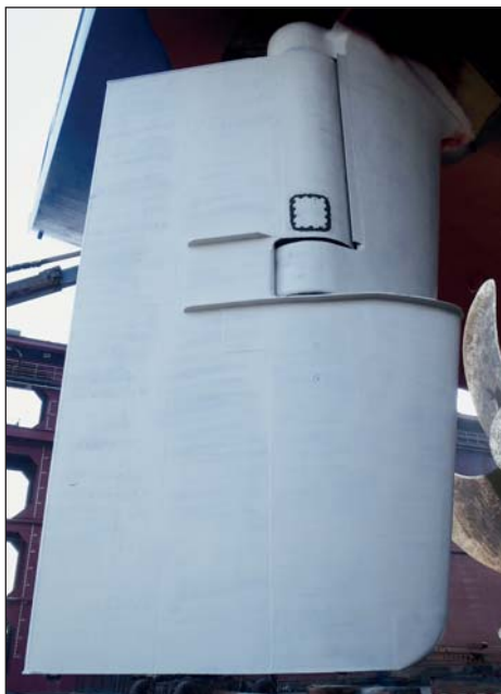
After surface preparation, Ecoshield is applied in two identical layers that will last for the ship's service life.
