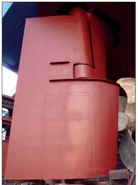
After surface preparation, Ecoshield is applied in two identical layers that will last for the ship's service life.
