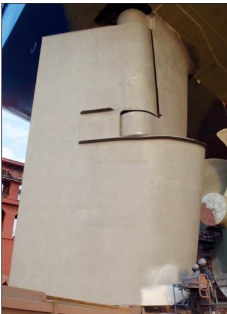
After surface preparation, Ecoshield is applied in two identical layers that will last for the ship's service life.
