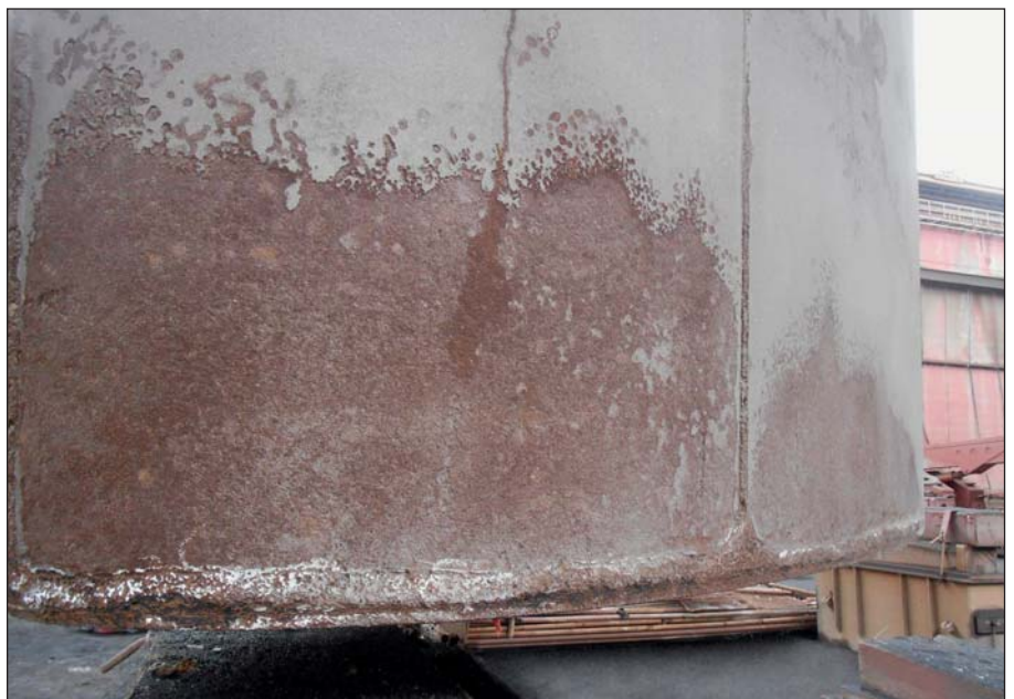
Cavitation and corrosion damage can destroy a rudder, so a lasting protection is essential.
