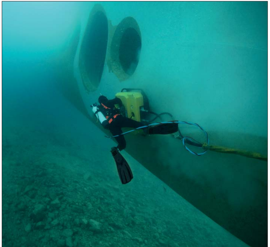
Underwater cleaning of Ecospeed can be carried out whenever needed, at any point in the coating's lifespan.
