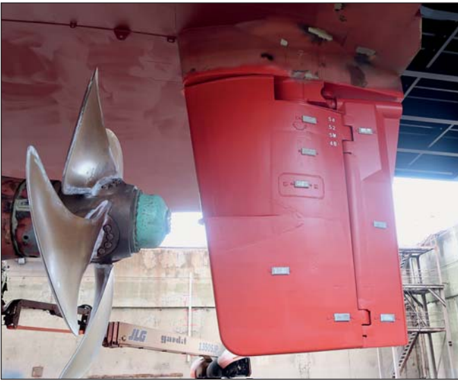
Rudder of roro vessel after Ecofix and Ecoshield combination has been applied.
