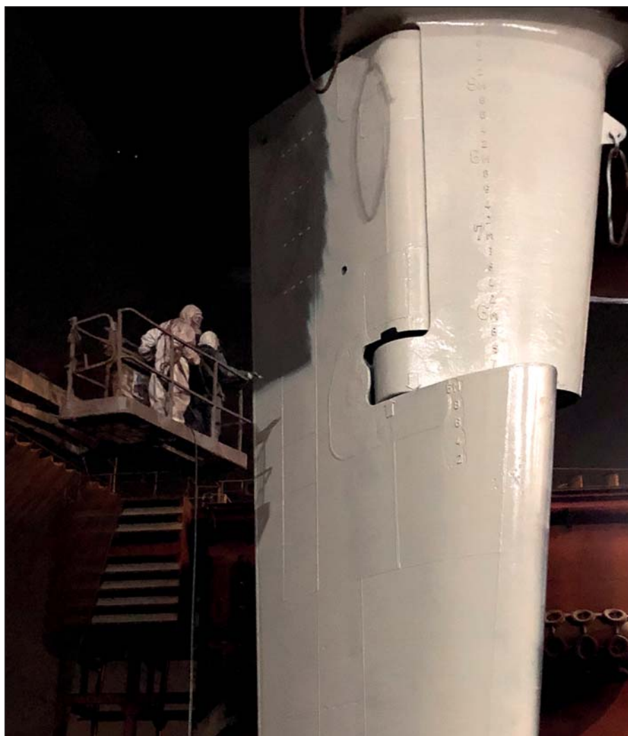
Application of first of only two Ecoshield layers.
