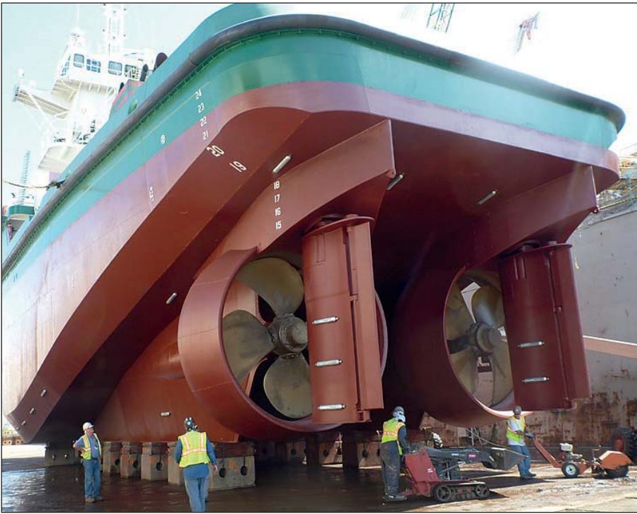
All types of nozzles can be safeguarded from cavitation and corrosion damage.
