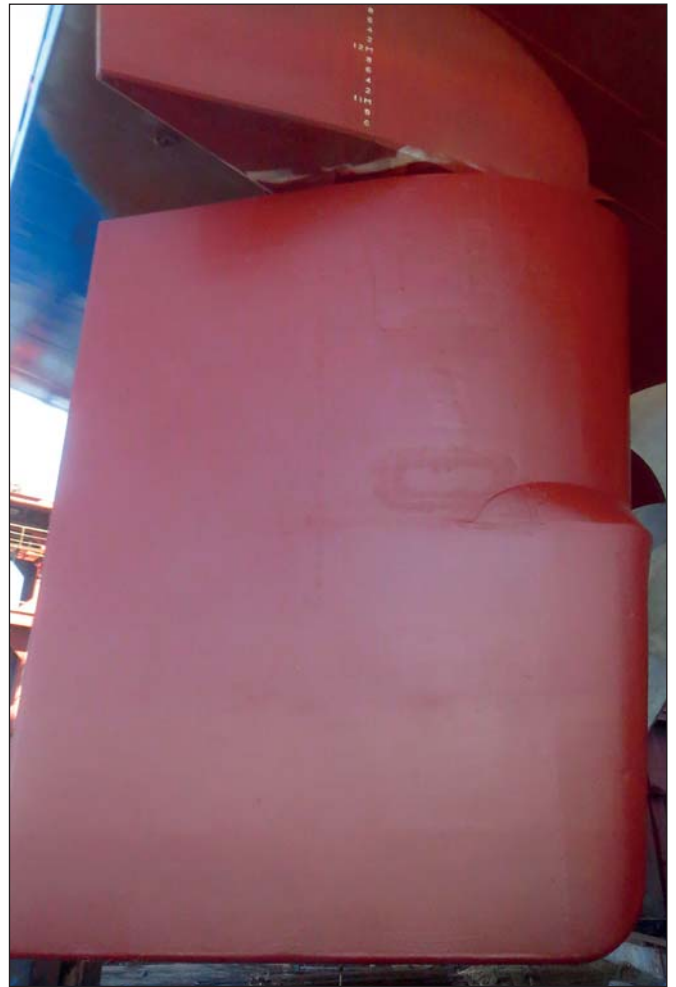
Ecoshield protects a rudder against cavitation and corrosion damage.
