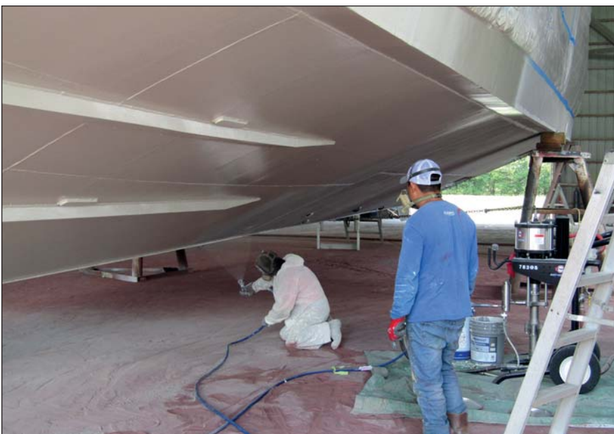
Application of first Ecospeed layer.
