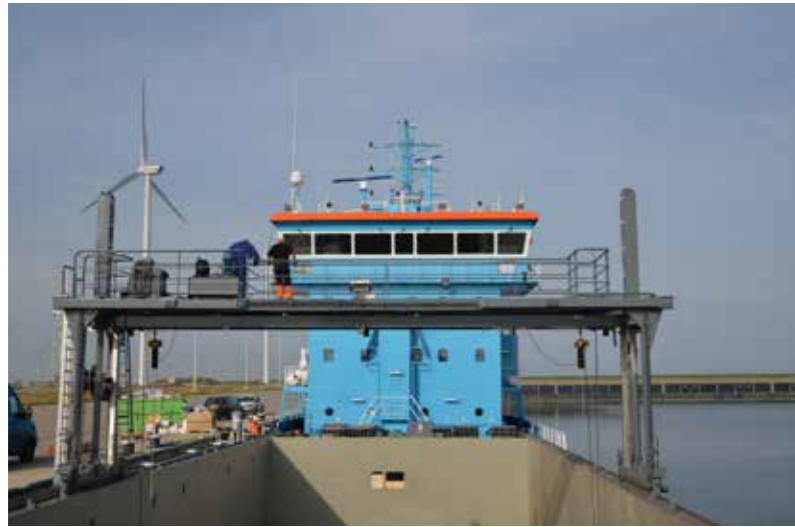
Handling of hatch and grain bulkhead panels is done with a gantry crane on coaming rails
