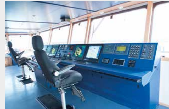
The wheelhouse forward area contains the T-shaped navigation console
