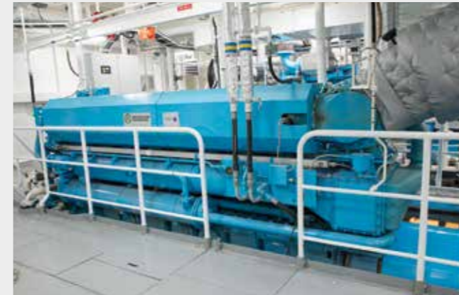
A multi-fuel medium speed 8-cylinder main engine is the heart of the EcoCoaster
