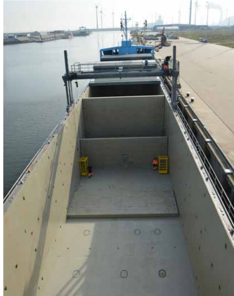
The tween deck panels can be positioned at a horizontal level or vertically, as bulkheads
