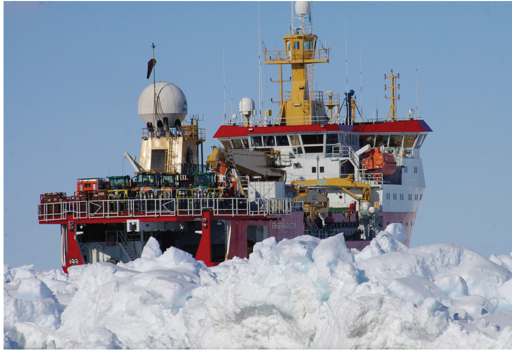
British Antarctic Survey ship Ernest Shackleton sailed in ice for four seasons with an Ecospeed coating that did not deteriorate
