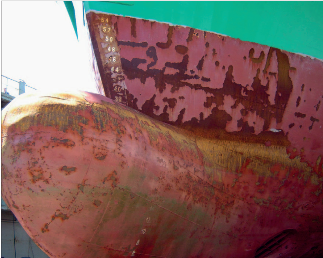
The hull of the ice-going MV Patriot: left – usual condition at drydock before Ecospeed application, and right – on return to drydock after 5 years trading in the ice with its Ecospeed coating.
