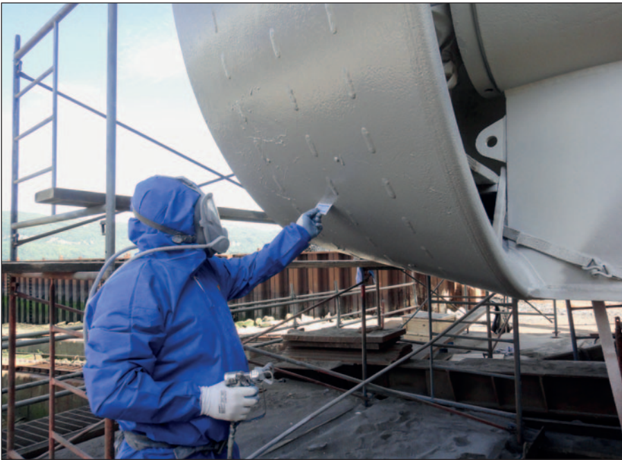
Applicator checking the wet film thickness on the Ocean Raymond Lemay.
