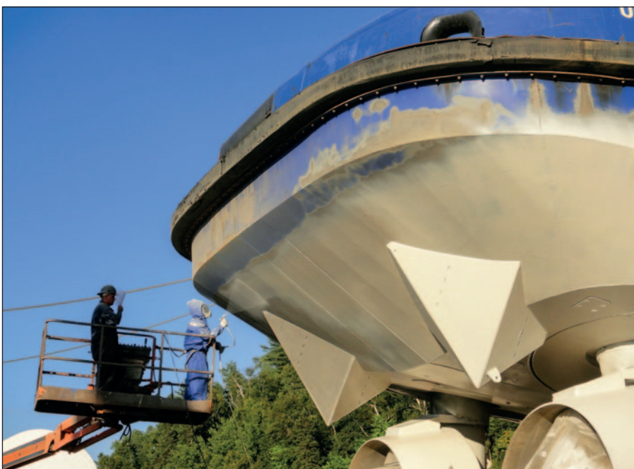
Ocean Raymond Lemay in January 2012, the first Ocean tug to be coated with Ecospeed Ice.
