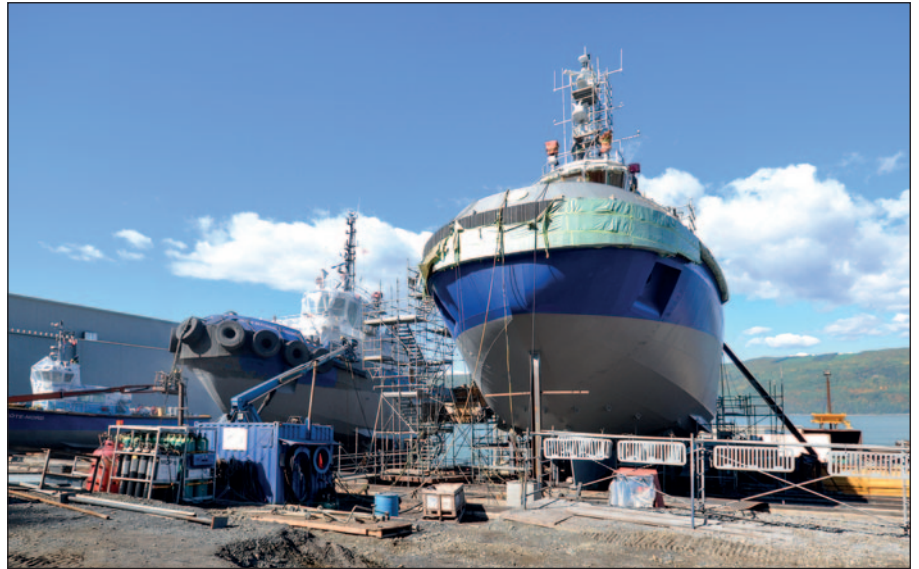
The Ocean TundRA 100 (right) in the Ocean Isle-aux-Coudres shipyard in Quebec, just painted with Ecospeed Ice in 2013.
