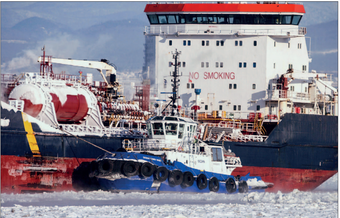
Ocean Henry Bain tug with Ecospeed Ice on the hull for full protection against the very harsh conditions of the St. Lawrence river and the Great Lakes.
