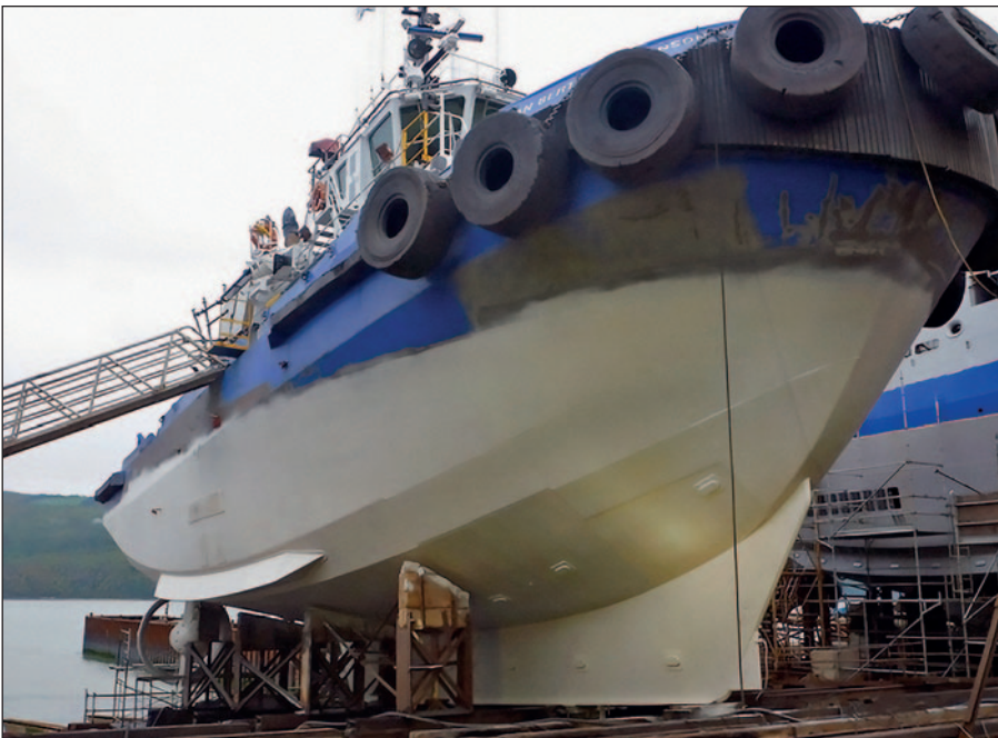
In 2013, the Ocean Bertrand Jeansonne's hull was coated with Ecospeed Ice.
