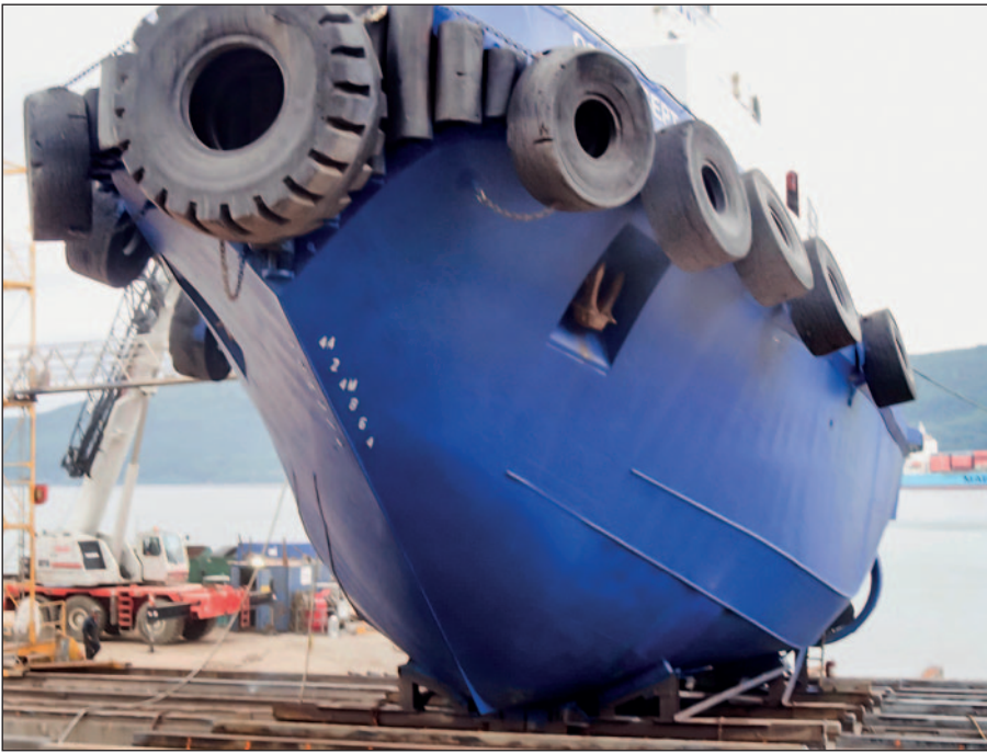
The Ocean Sept-Isles in drydock three years after Ecospeed Ice was applied.
