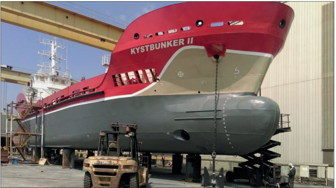
Oil tanker after application of second Ecospeed layer in shipyard in Turkey.
