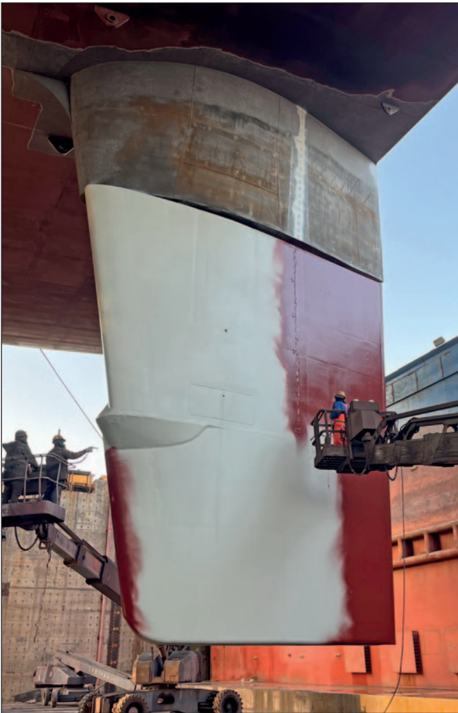
Ecoshield has been designed to give a very thorough and lasting protection against cavitation damage and corrosion.
