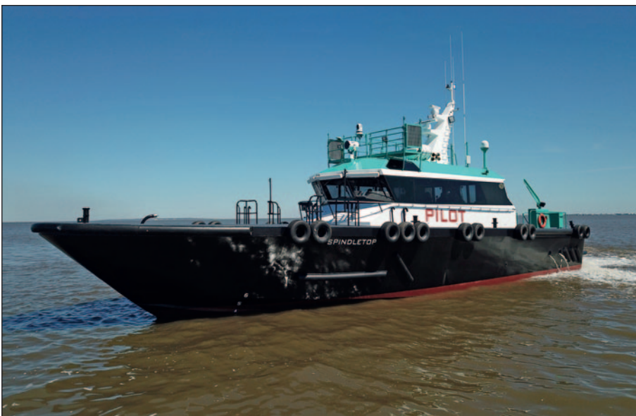
Spindletop is the largest aluminum pilot boat constructed in the US. The boat was coated with Ecospeed in 2021.
