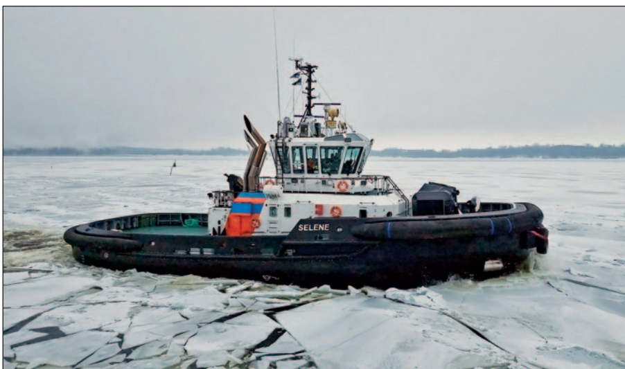
This icebreaking tugboat has been protected by Ecospeed ice since it was built.
