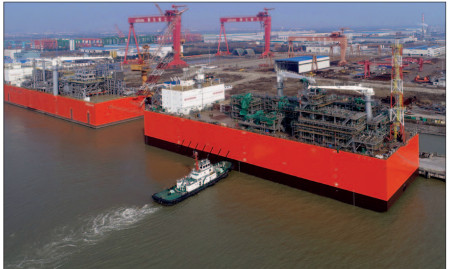
Floating Storage and Regasification Unit (FSRU) during its undocking.
