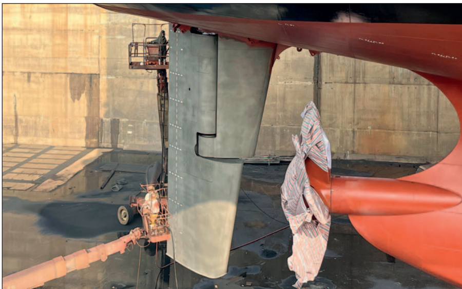
After grit blasting, the rudder is ready for Ecoshield application.
