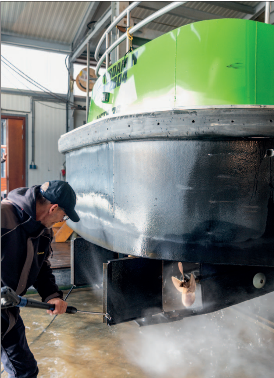
Regularly pressure washing the Ecospeed-coated hull of a water taxi in Rotterdam ensures top fuel performance.
