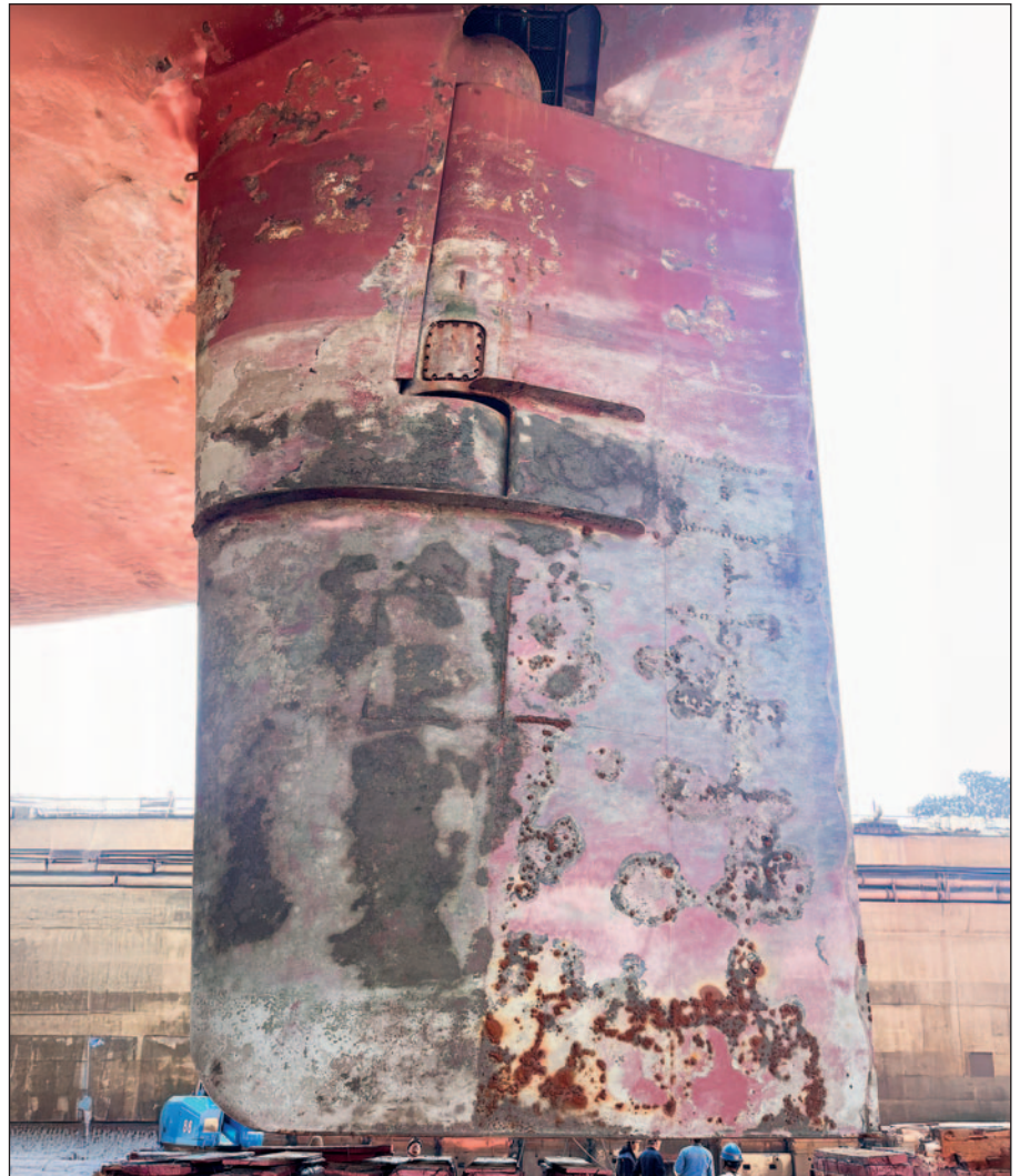
Corrosion and cavitation damage can have a devastation effect on rudders if they are not given the proper protection.
