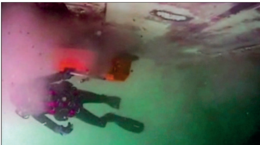
Trying to clean a hull with an antifouling coating harms the coating and the marine environment.
