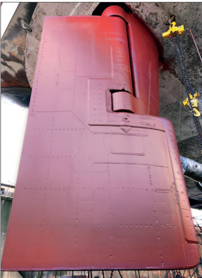
No anodes are required on rudders coated with Ecoshield.
