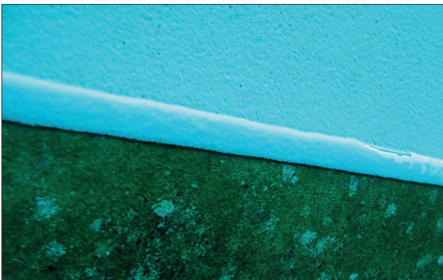
Ecospeed allows for complete removal of extensive fouling through underwater cleaning after extended layup periods with the coating always intact.
