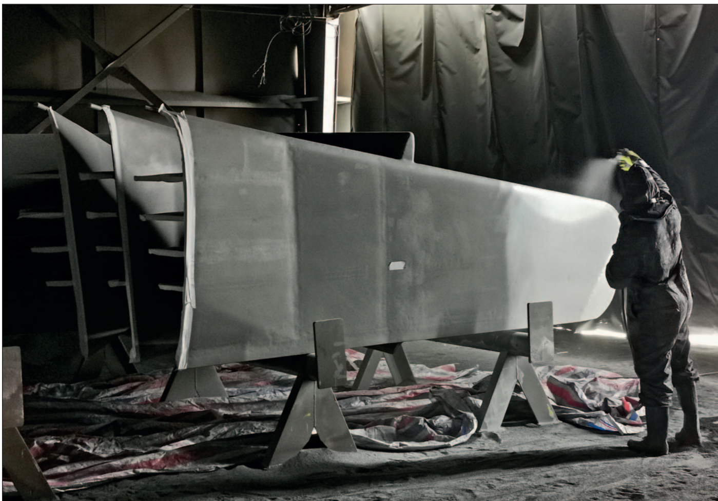
Ecoshield can be applied prior to installation of the rudder gear.
