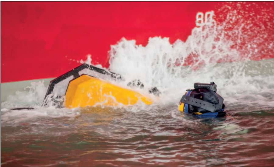
Cleaning a cruise ship hull protected with Ecospeed is a simple task.
