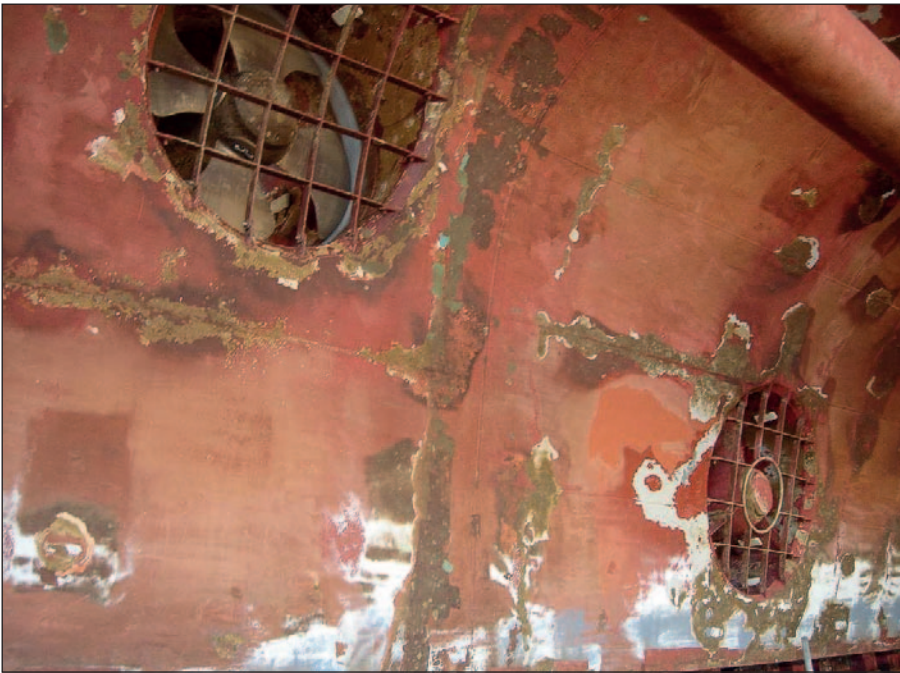
Cruise ship hull after 5 years of sailing with a traditional antifouling coating scheme.
